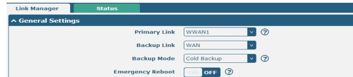
Link Settings section allows user to configure the parameter of link connection, include the WWAN1/WWAN2, WAN and WLAN. It is recommended to enable Ping detection to keep router always online. The
